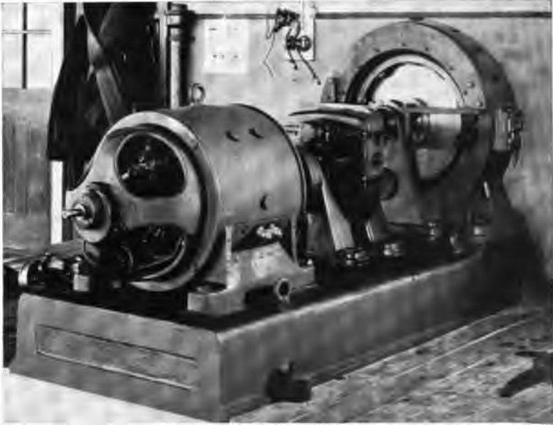
FIG. 197.—Experimental high-frequency generator at Siemens' Works, Woolwich (1912).
